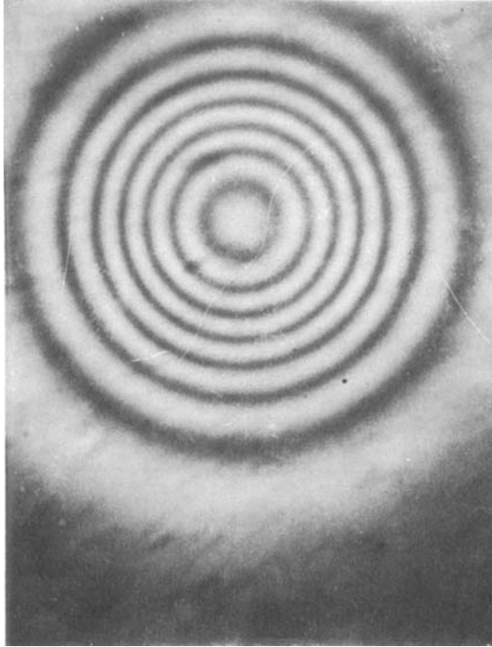
FIGURE 3. Interference fringes formed by reflection of red light on a deposit of tungsten oxide.
